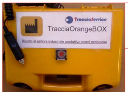
The device is a box of dimensions 29x22,5x8cm, supplies through the taking of the car lighters and, in case of need, form an inside battery that allow it an autonomy of 36h.
